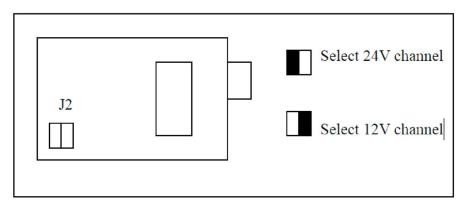
Note: J2 is used to select the voltage source from mother board. Actually, the 12V or 24V is the name for distinguishing these two channel. You can input voltage of 8~24V to V12 or V24 terminals of mother board.
